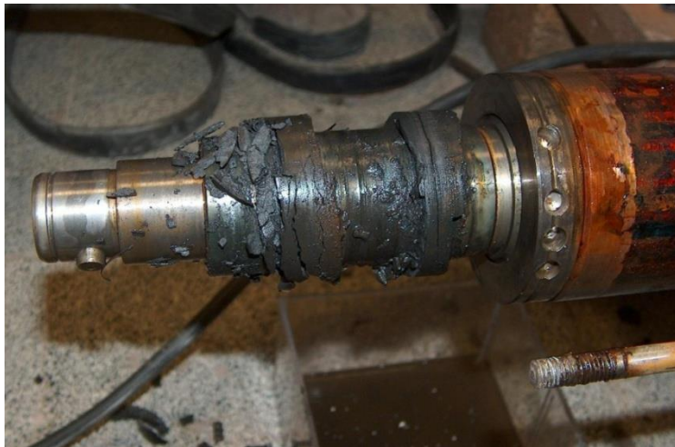
Destruction of motor journal bearings shaft
