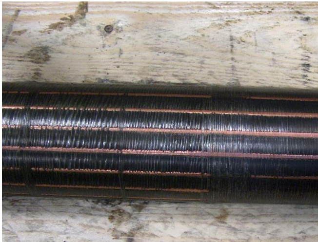
Destruction of motor journal bearings shaft
