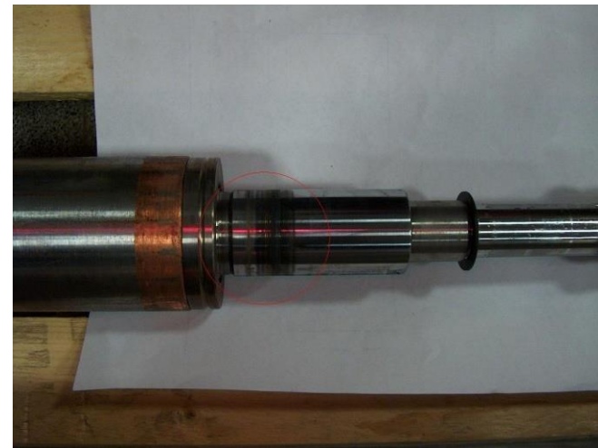
Destruction of motor journal bearings shaft
