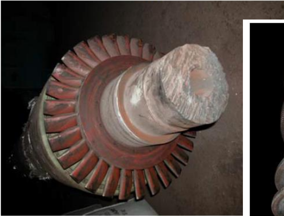
Destruction of generator shaft
