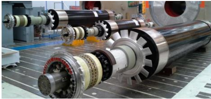
Picture 1. Generator rotor by BRUSH (www. brush. com)
